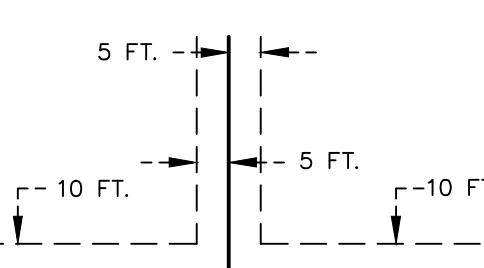
BEING 5 FEET IN WIDTH ADJOINING SIDE AND REAR LOT LINES, AND BEING 10 FEET IN WIDTH ADJOINING PUBLIC WAYS UNLESS OTHERWISE INDICATED ON THIS PLAT
