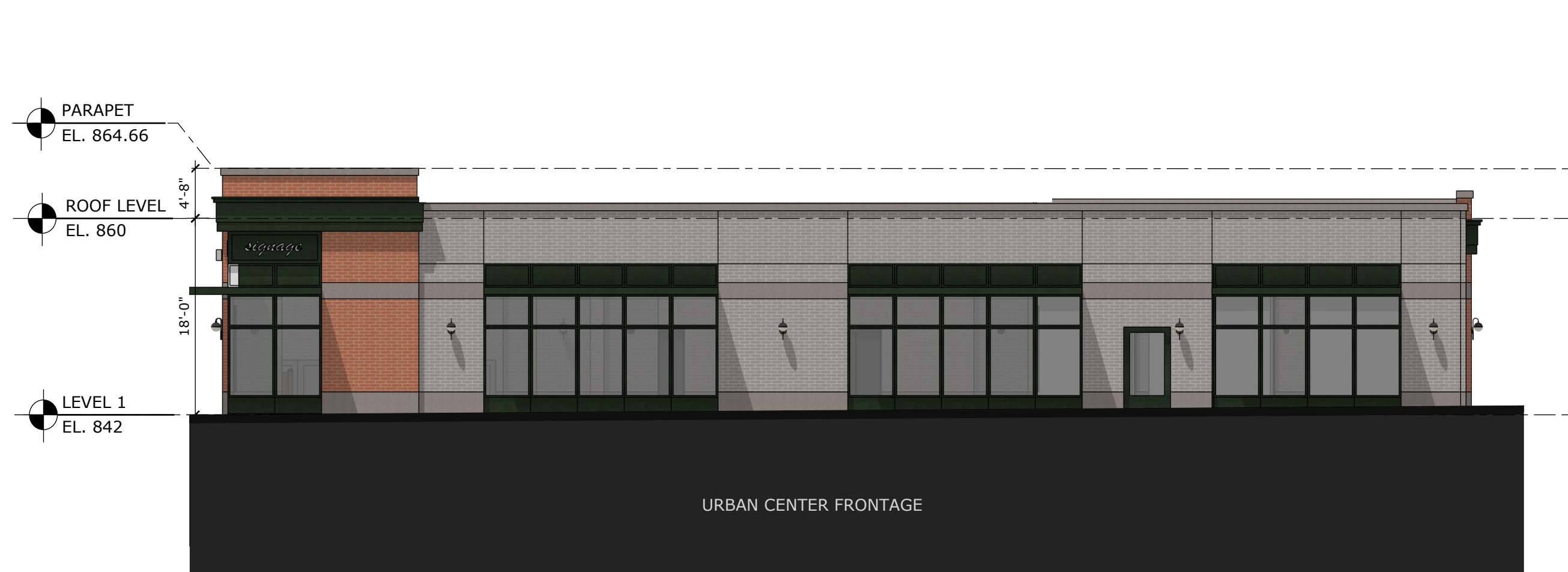
3 BLOCK 2C - EAST ELEVATION SCALE: 3/32" = 1'0"
