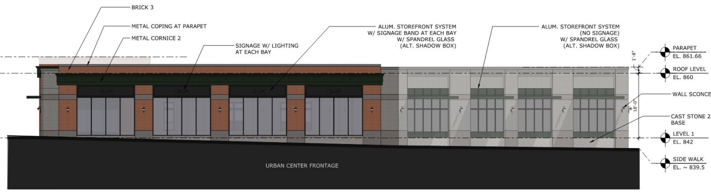
4 BLOCK 2c - NORTH ELEVATION SCALE: 3/32" = 1'0"
