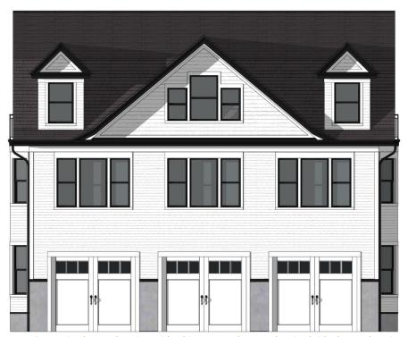
Image 10c - Revised Rear elevation with white garage doors and revised side dormer locations.
