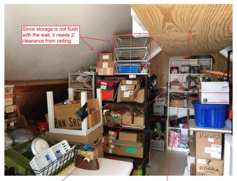
Note, storage which is flush with the wall can go to the ceiling. So there is no code concern with the white shelving unit.
