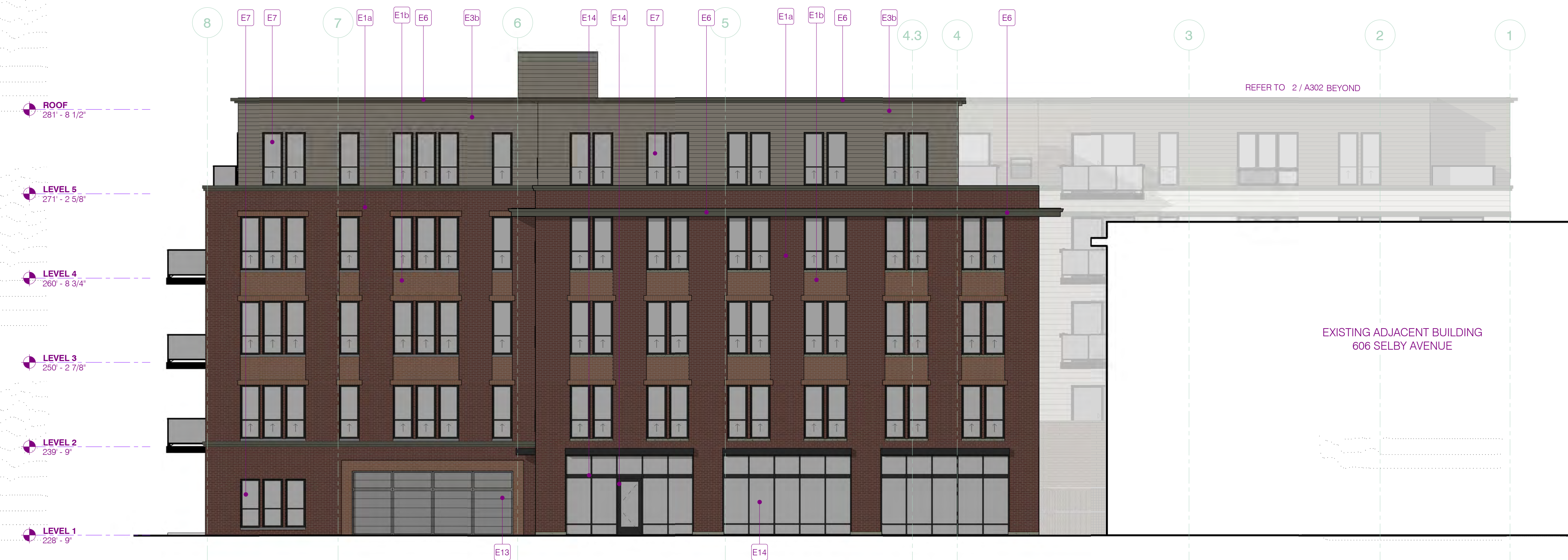
1 NORTH ELEVATION (SELBY) A301 1/8" = 1'-0"
