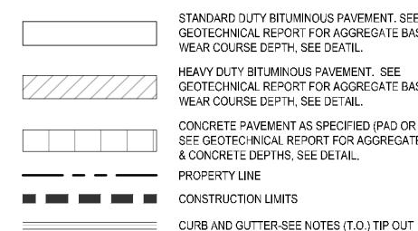
STANDARD DUTY BITUMINOUS PAVEMENT. SEE GEOTECHNICAL REPORT FOR AGGREGATE BASE &
