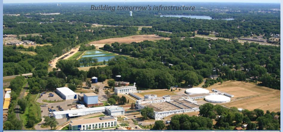
\$130M Design-Build Water Treatment Improvement Project which includes process improvements in softening, recarbonation, and ozone disinfection.
