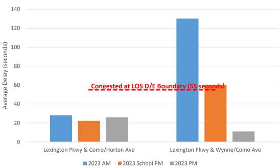
Chart 1 – Peak Hour Delays: Signal Controlled Intersections
