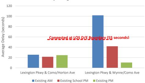
Chart 1 – Peak Hour Delays: Signal Controlled Intersections
