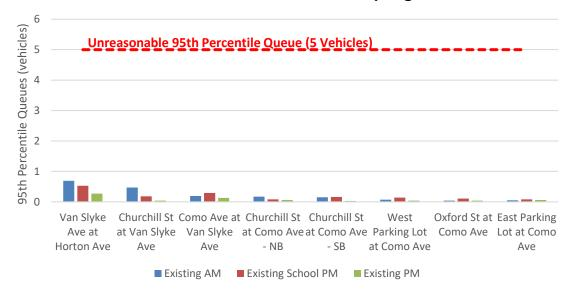
As shown in Charts 1 and 2, most study intersections and movements are operating acceptably in the existing peak hours. These computer results match the magnitude of delays and vehicle queues observed in the field.
