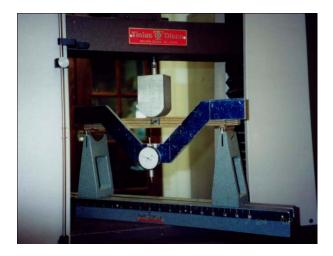
Our in-grade full size lumber testing machine is used to evaluate lumber in bending as well as in tension. Materials from 2"x 4" x 8' up to 2"x 10"x 16' sizes can be evaluated. All data is recorded using a data acquisition system.
