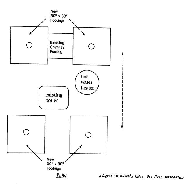
NOTES: Each footing to be 30"x30"x. deep, with three #4 rebars evenly spaced in the N/S and E/S directions, for a total of six rebar per footing. Existing posts are to be replaced with permanent structurally code approved steel posts. A new plinth block is needed under the next post south of the existing chimney.
