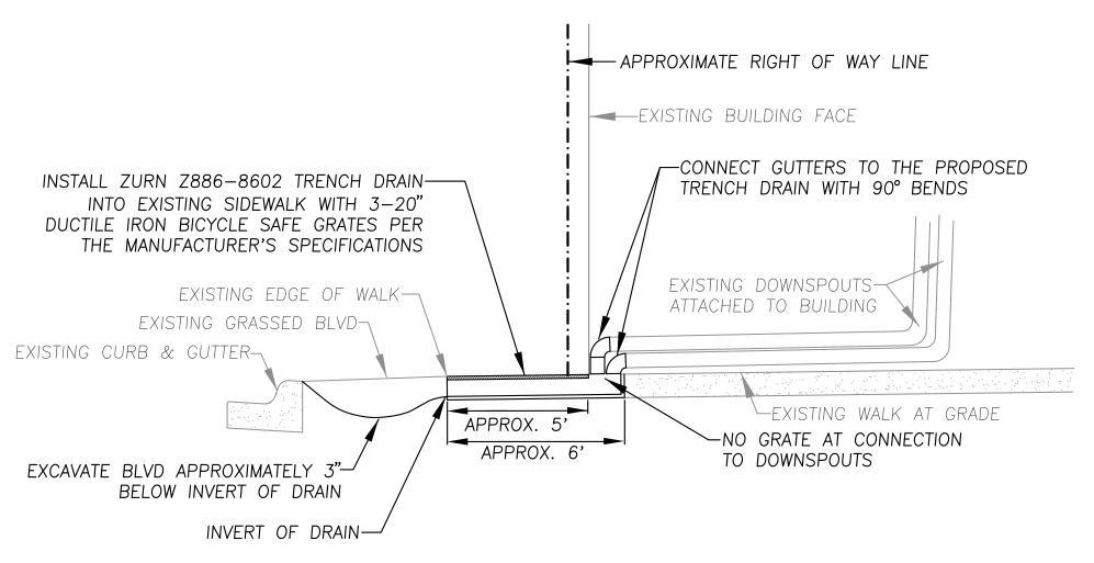
NOTE: REPAIR CONCRETE AS NEEDED MATCHING EXISTING PAVEMENT SECTIONS.
