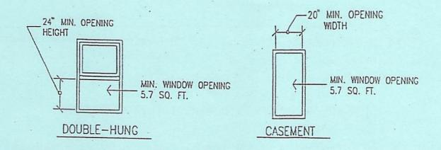
NOTE: 5.7 SQUARE FEET = 821 SQUARE INCHES WHEN MULTIPLYING WIDTH TIMES HEIGHT OF THE OPENING IN INCHES.
