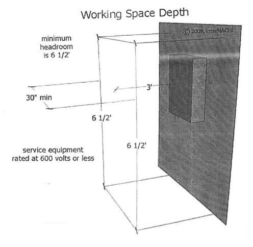
Minimum width of working space is the width of the equipment or 30 inches, whichever is greater.
