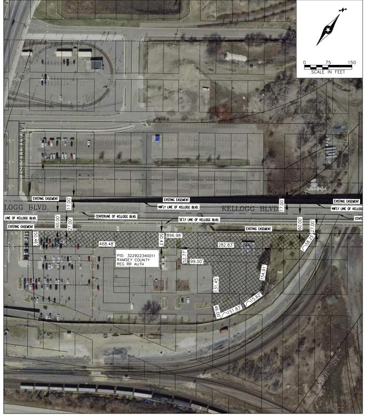
**ADDRESS** PID PARCEL LINE EXISTING R/W EXISTING PE 322922340011 **EXISTING** PERM EASE (PE) [SQ.FT] TE [SQ.FT] TEMP EASE PROPOSED PE CONST LIMITS TREE REMOVAL RAMSEY COUNTY **PARCEL** REG RR AUTH AREA [SQ.FT] ŏ 222788.94 SQ FT 0.00 SQ FT 83216.57 SQ FT TREE W/IN TEMP EASE KELLOGG/3RD ST. BRIDGE REPLACEMENT
