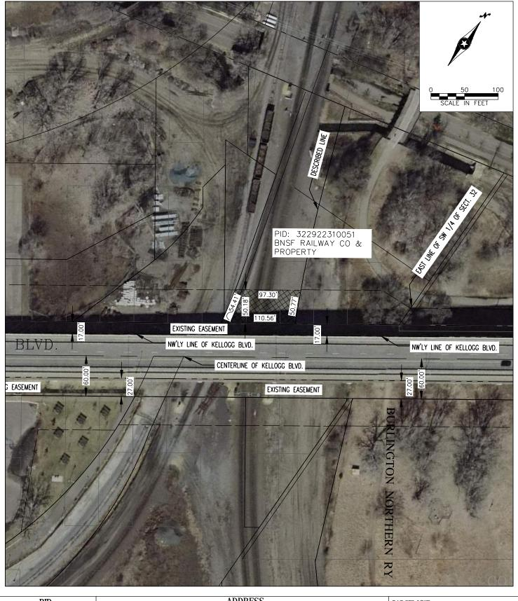
ADDRESS PID 322922310051 **EXISTING** PERM EASE (PE) [SQ.FT] TE [SQ.FT] BNSF RAILWAY CO PARCEL AREA [SQ.FT] & PROPERTY 36710.60 SQ FT 0.00 SQ FT 5192.71 SQ F
