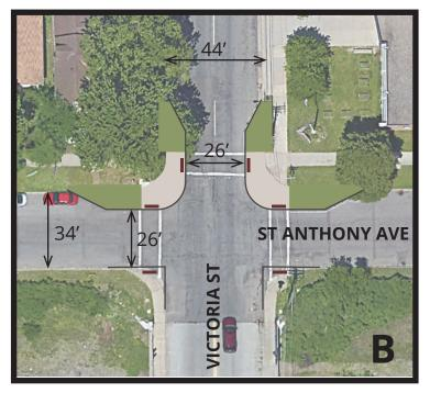
Location B. Install curb extensions on NE and NW corners to narrow N, E, W crossings to approx. 26'.
