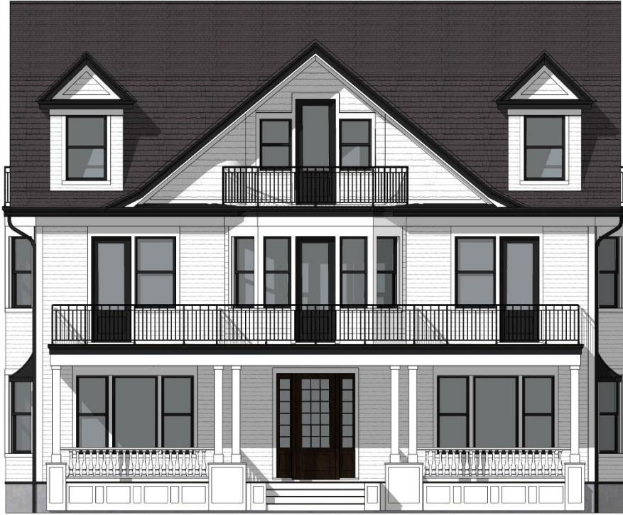
Image 10b - Revised front elevation with revised location of side dormers (12" towards the center).
