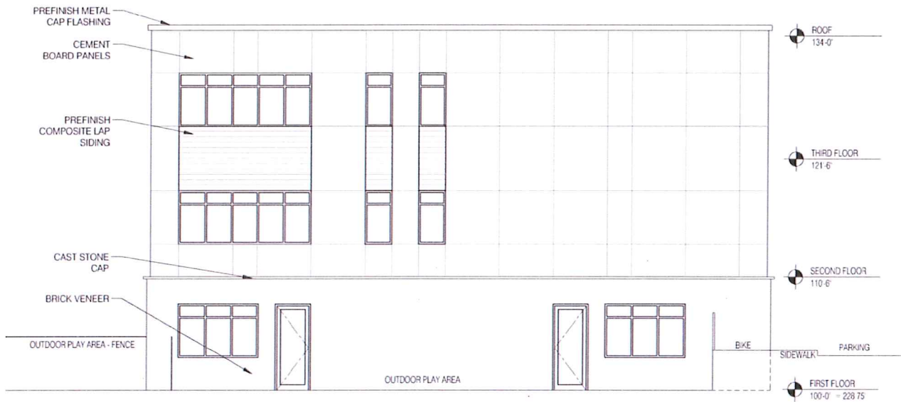
1 WEST ELEVATION A1.5 1/8"-1'-0"
