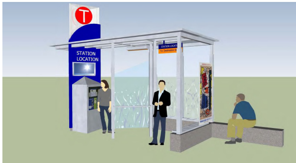
Small transit station with windscreen concept, rapid bus Source: Metro Transit Arterial Transitway Corridors Study
