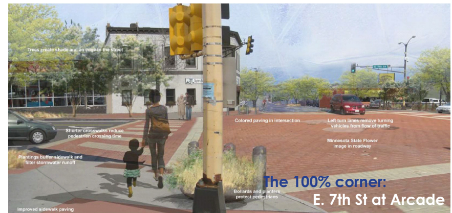
Possible improvements at intersections include improved sidewalk paving, bollards and planters to increase pedestrian safety, plantings to buffer pedestrians and filter stormwater, shorter crosswalks to reduce pedestrian crossing times, and colored paving and a meaningful image printed in the middle of the intersection
