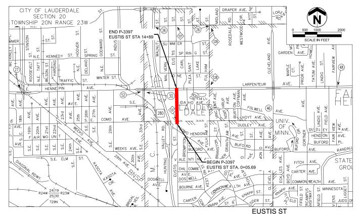
ADT (CURRENT YEAR) 2025 \_\_3130 ADT (DESIGN YEAR) 2045 3600 DHV (DESIGN HR. VOL.) (DIRECTIONAL DISTR.) 59% (HEAVY COMMERICAL) 3.98% SOIL FACTOR R-VALUE TON DESIGN
