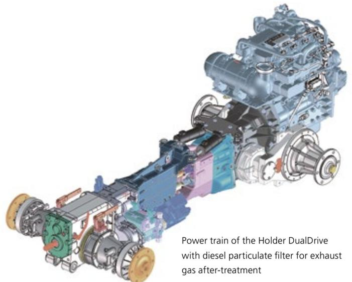
Power train of the Holder DualDrive with diesel particulate filter for exhaust gas after-treatment
