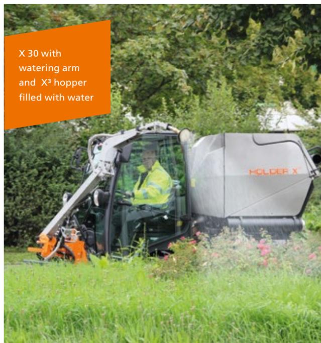
X 30 with watering arm and X<sup>3</sup> hopper filled with water
