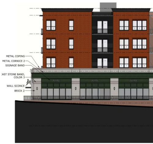
4 NORTH ELEVATION SCALE: 3/32" = 1"
