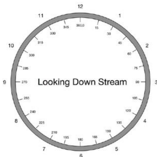
Figure 3 – Clock Reference for Recording Observations.
