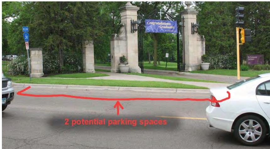
Next to the Accolades Spa 15-space parking lot, is an unused driveway that can provide an additional 2-space parking bay. It is currently useable as-is but could be officially signed and proper curb-cuts added at a later date. This would make up for an additional 2 of the 9 lost parking spaces.
