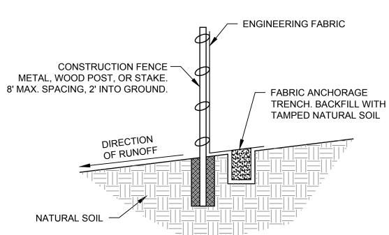
NOTE: DEPENDING UPON CONFIGURATION, ATTACH FABRIC TO WIRE MESH WITH HOG RINGS, STEEL POSTS WITH WIRES, CONSTRUCTION FENCE WITH WIRES, OR WOOD POSTS WITH STAPLES.
