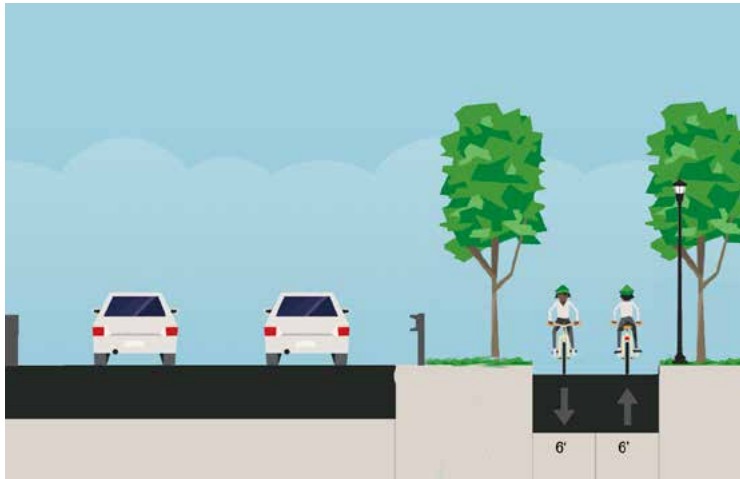
Figure 24: Segment 4 typical section. 12'-0" trail to replace existing 8'-0" trail, new vegetation buffer & pedestrian lights.
