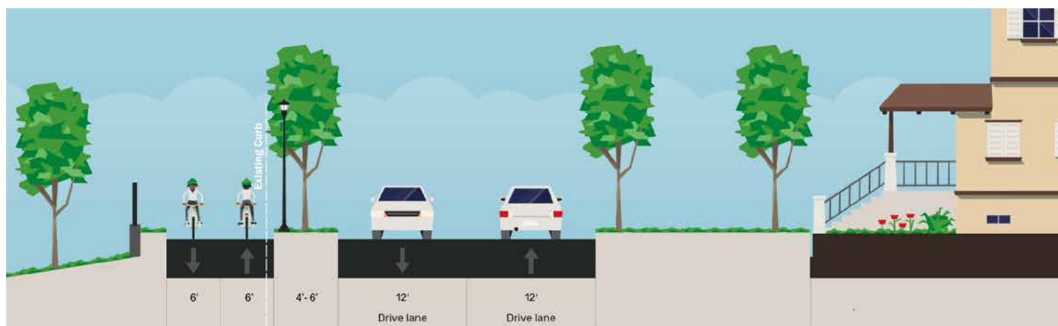
Figure 19: Segment 3A typical section.
