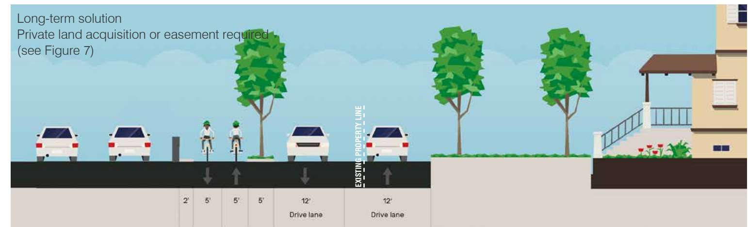
Figure 22: Segment 3B grade separated trail along Point Douglas Rd between Highwood Ave and Howard Ave.
