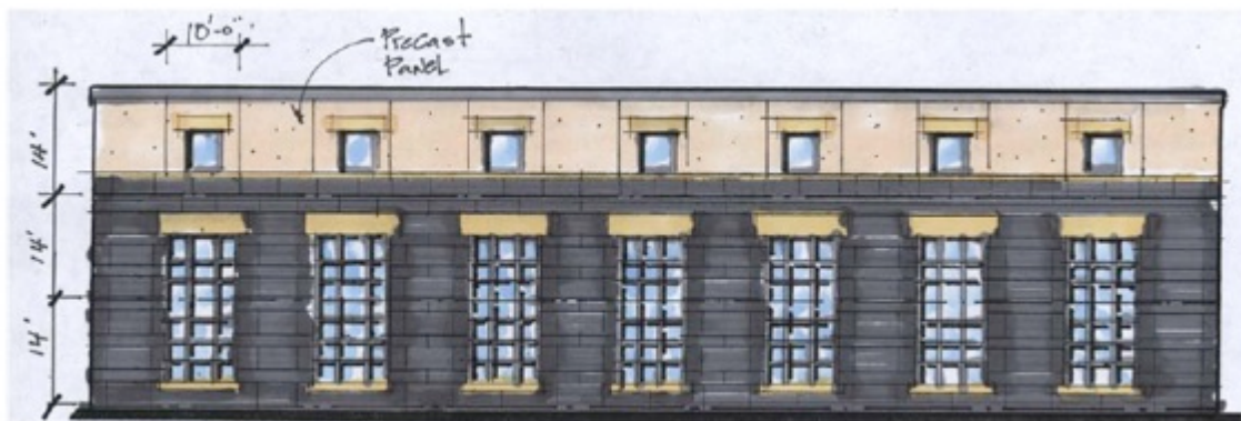
Figure 3: 42' tall by 150' long vertical wall adjacent to residential parcel. Zoning allows this elevation to be located 12'-0" away from adjoining homes. Mechanical equipment on the roof will increase this mass.
