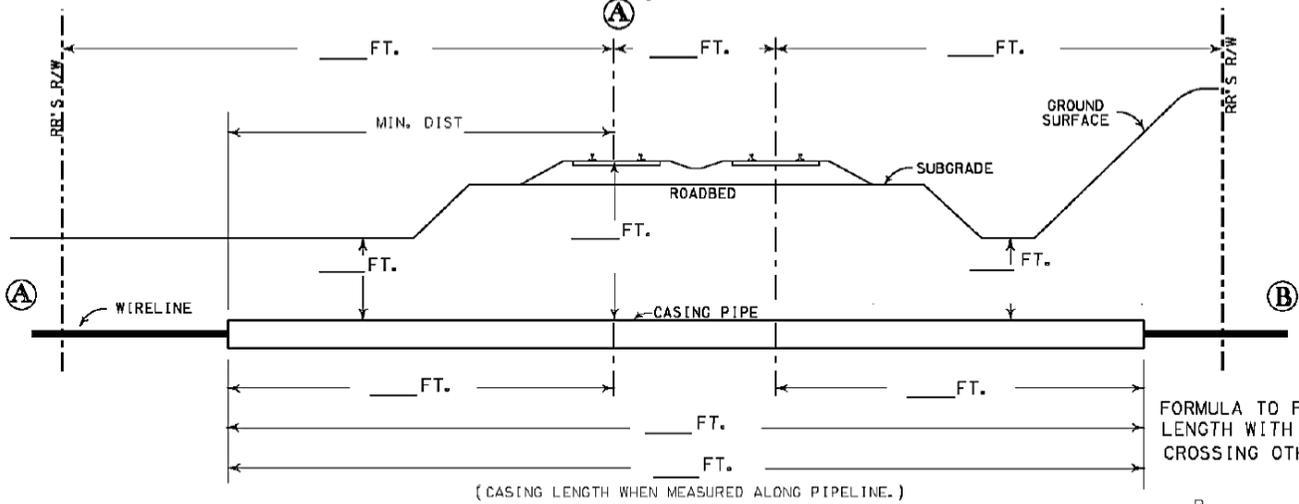
FORMULA TO FIGURE CASING LENGTH WITH ANGLE OF CROSSING OTHER THAN 90°
