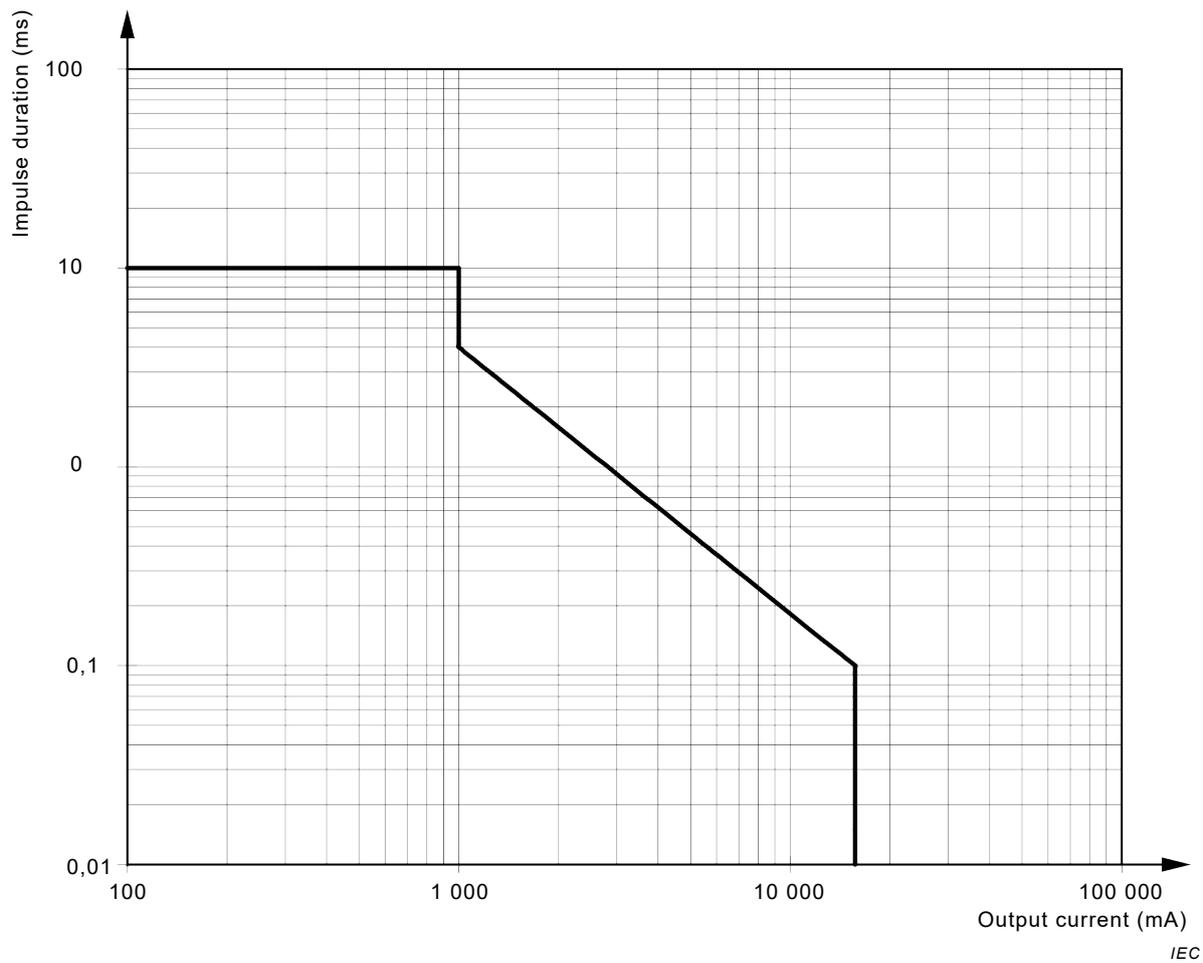
NOTE The equation of the line relating **impulse duration** (ms) to **output current** (mA) for  $1\,000\text{ mA} < \text{output current} < 15\,700\text{ mA}$ , is given by  $\text{impulse duration} = 41,885 \times 10^3 \times (\text{output current})^{-1,34}$ .
