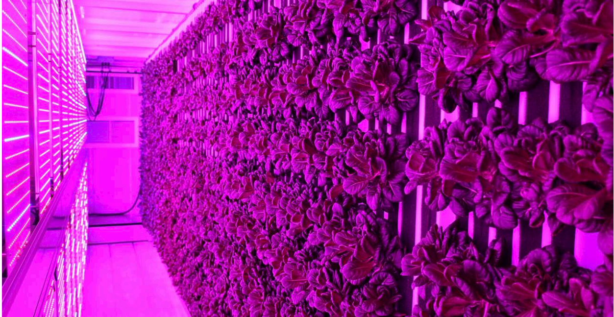
Figure A3: True color image of the “Greenery” farming system in operation. The red and blue LED light banks deliver photons of specific energies that catalyze the red and blue chlorophyllic reactions, resulting in the overall pink illumination. Notice the hundreds of healthy plants which grow in the vertical rows of each growing rack. The “Greenery” system can enable an astounding 8,800 living plants to grow within at a given time. Image drawn from the website of the manufacturer, Freight Farms ( www.FreightFarms.com ).
