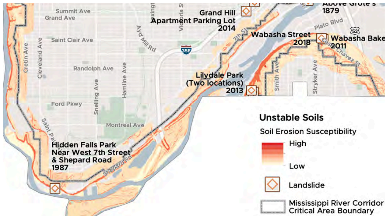
Fig. 5. Map CA-8 of the MRCCA Publication, showing unstable soils as measured by soil erosion susceptibility. South Campus is in upper left.
