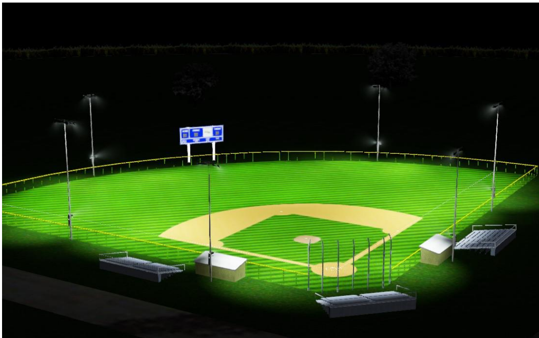
Examples of recreational lighting technologies that focus lights downward on the fields and limit light spill across property lines
