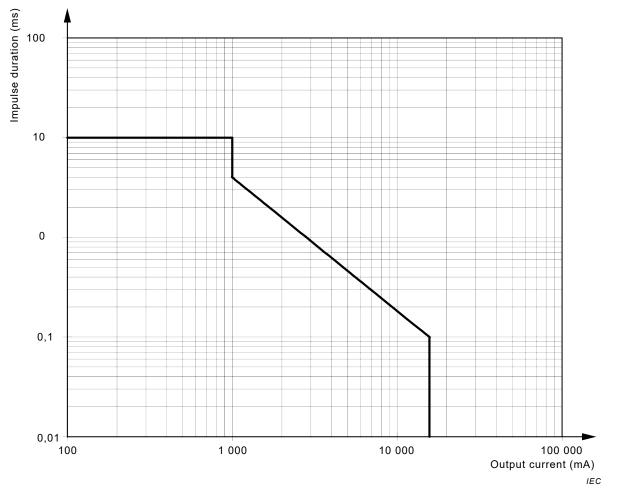
NOTE The equation of the line relating impulse duration (ms) to output current (mA) for 1 000 mA < output current < 15 700 mA, is given by impulse duration =  $41,885 \times 10^3 \times (output current)^{-1,34}$ .
